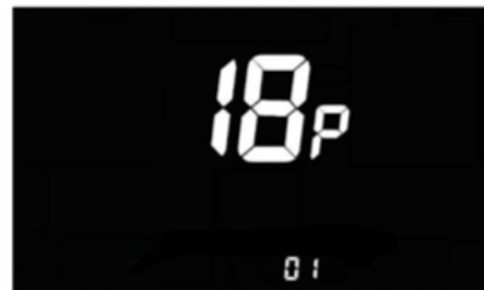
Figure 6-18 6km/h walk boost setting interface
