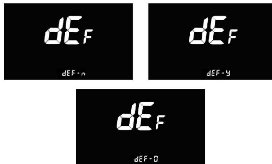
Figure 7-1 Restore factory default parameter setting interface
