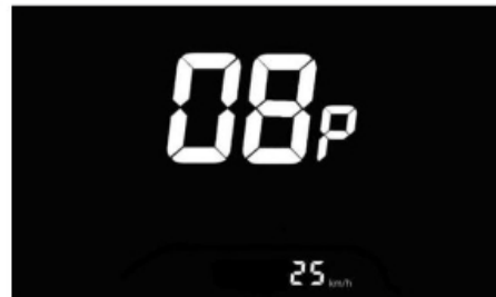
Figure 6-8 Speed limit setting Interface
