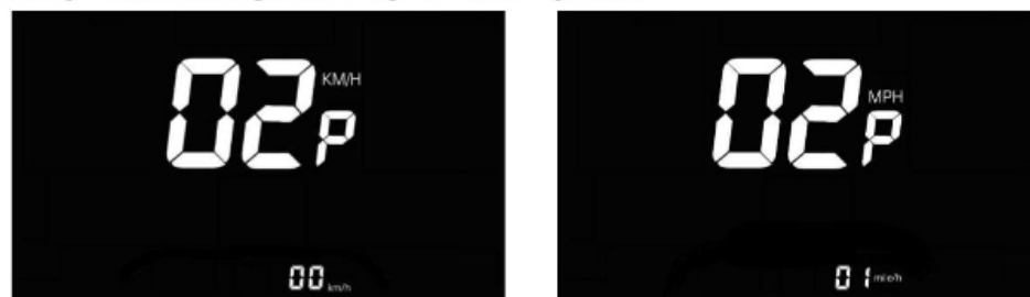
Figure 6-2 Metric and Imperial setting interface
