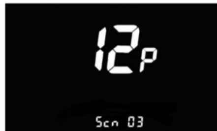
Figure 6-12 Pedal assist strength setting interface
