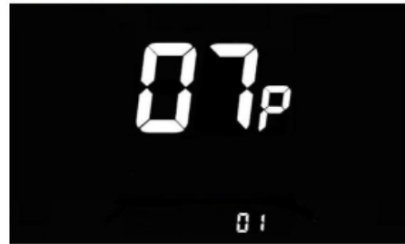
Figure 6-7 Number of speed sensor magnets setting Interface
