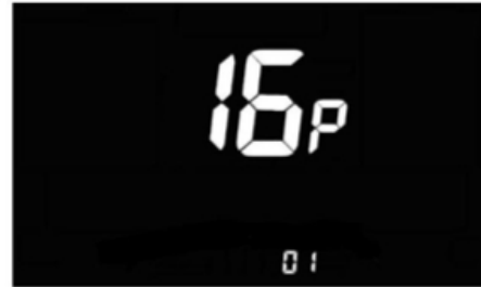
Figure 6-16 ODO reset setting interface
