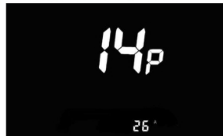
Figure 6-14 Controller current limit setting interface
