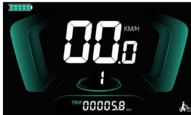
Figure 5-2 Walk boost mode display interface
