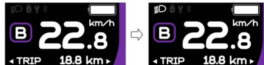
Headlight switch interface
