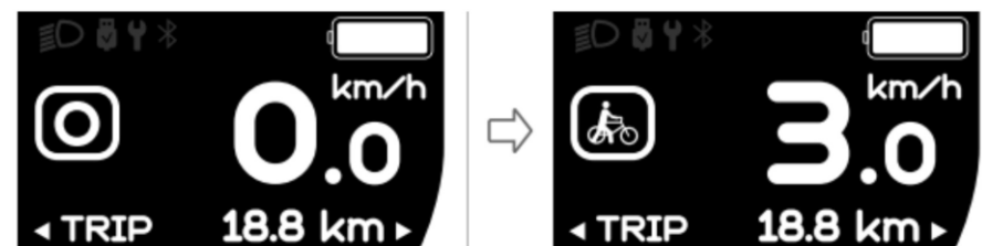
Power-assisted push mode switching interface
