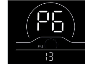
Fig. 4-6 Current Limit Setting Interface
