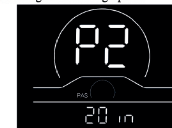
Fig. 4-2 Wheel Diameter Setting Interface
